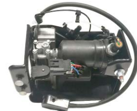
CD-7760 AIR COMPRESSOR
